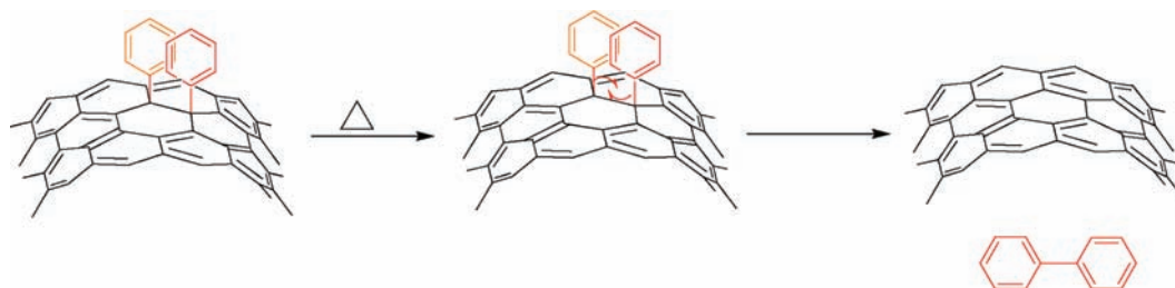
Scheme 1. Proposed Mechanism by Margine et al. for the Detachment of Phenyl Addends from the SWNT Sidewall a
